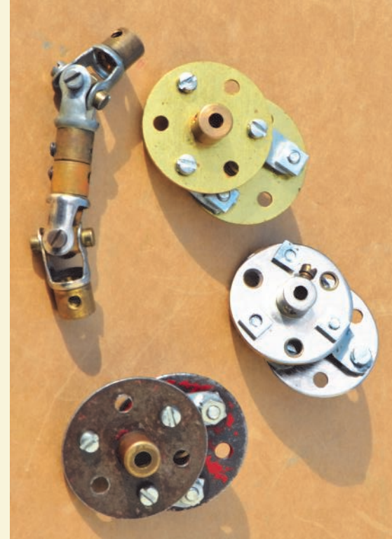
Jim Osborne's hole spacer and Doug Ward's universal coupling alternative
